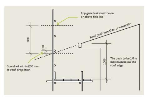
A scaffold platform may be positioned to provide roof edge protection. The picture shows the location of the scaffold platform when scaffolding is used to provide guardrailing for roof work when the roof pitch is 25 degrees or less. To minimise the risk of serious injury from falling onto a scaffold platform from the edge of the roof, locate the platform as near to the gutter line as possible and no more than one metre below the lower edge of the roof surface.
